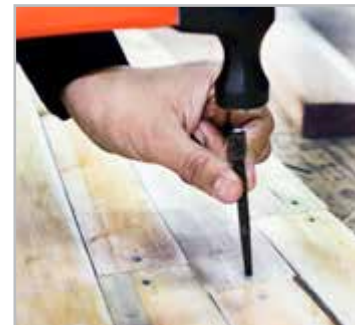
The working end is cupped to follow the nail head without sliding off
