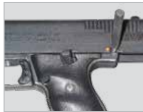
Roll Pin Punch being used to remove spring pin from a gun
