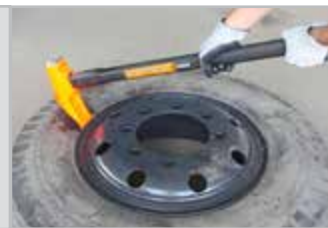
Convex shaped wedge penetrates the tyre bead & loosens it
