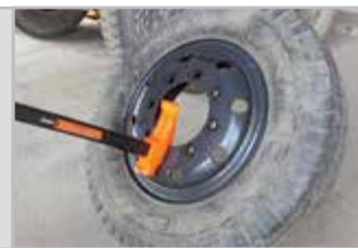
Convex shaped wedge penetrates the tyre bead & loosens it
