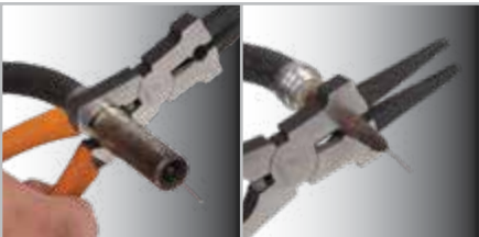
Nozzle removal & installation
