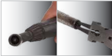
Welding Gun Nozzle filled with weld splatter
