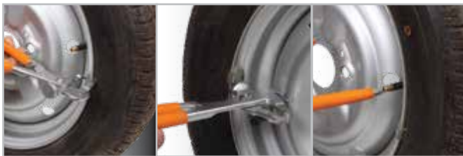
Plier being used to detach wheel balancing weights
