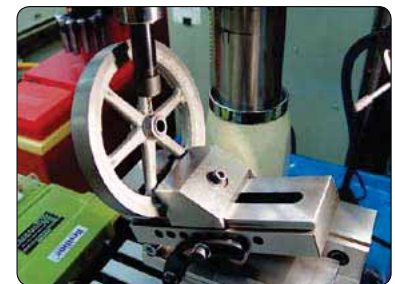
Sine Vice being used to drill an angled hole on a machine wheel
