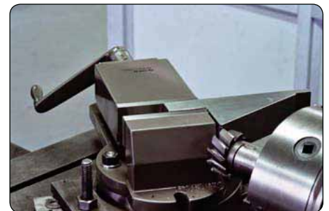
Milling machine vice being used to hold a job for milling operation
