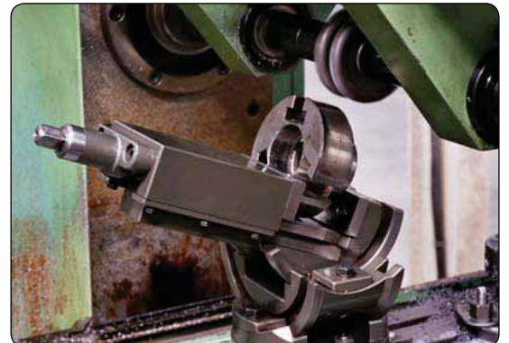
ThreeWayTiltingVice being used to hold a job at an angle for milling operation.
