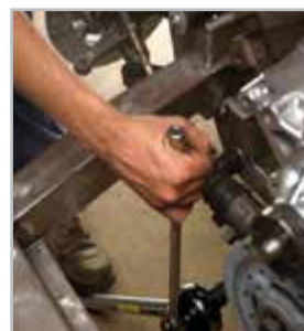
Torque multiplier used in inaccessible areas
