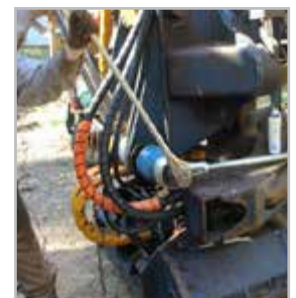
Torque multiplier used for machine nut tightening
