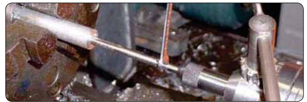
The concave end is good for smaller taps, which usually have a 60° taper ground at the end. This allows great support and alignment
