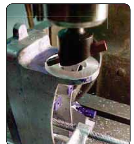
Fly Cutter Holder with tool being used for face machining of a job on a vertical milling center
