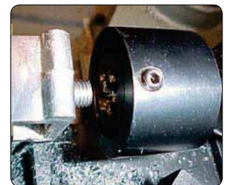
Die Holder holding a die being used for external thread cutting
