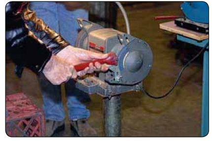
Dressing the wheel of a Bench Grinder
