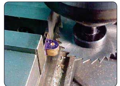
Slitting Saw Arbor being used for a slitting operation on a job being worked upon on a milling machine
