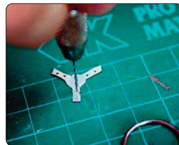
PinVice being used to hold a drill for hand-drilling on an electronic component
