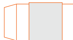
Screw on cap is used to hold and interchange collets
