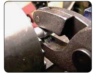
Knurling Tool Holder - being used for doing knurling on a job fitted onto a lathe machine
