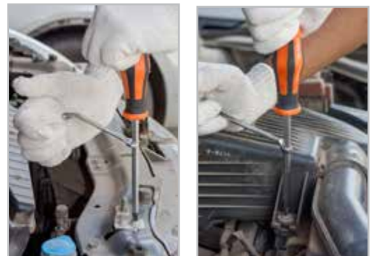
Hex shaft can be tightened using a spanner for high torque applications
