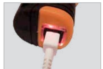
Red light show charging on & Green light shows charging complete
