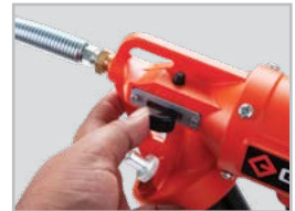
Slide backwards for Continuous Mode
