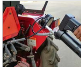
Without Swivel - Twisting of hose
