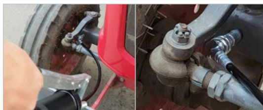
Convenient access into narrow, inaccessible greasing joints
