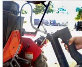
With Swivel - No Twisting of hose
