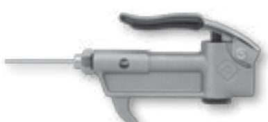
TYPE: N1 ss needle 1-3/4" (44 mm) long x 0.072" (1.8 mm) dia.
