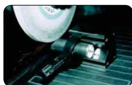
Non Protruding Clamp Type Vee Block used on side face for holding round bar in a grinding operation
