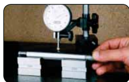
Regular Vee Block set used as an inspection tool for checking run-outs
