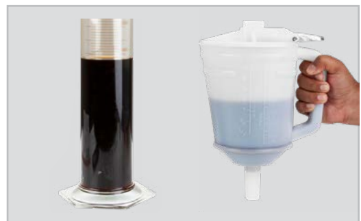
Measured quantity of oil transferred using the funnel
