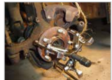
3 Jaw Puller used for removing tyre hub
