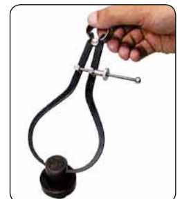
Outside Caliper being used to inspect the external diameter of a machined component
