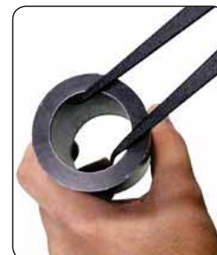
Inside Caliper in use to measure the internal diameter of a cylinder
