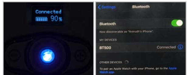
To activate Bluetooth, press and hold the ON button for switching on the Bluetooth mode and connect to "BT500" from your phone
